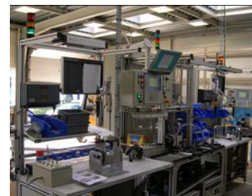
Line of hand-operated assembly of pumps
